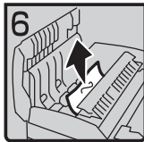
6. Remove the misfed original and close the cover.
